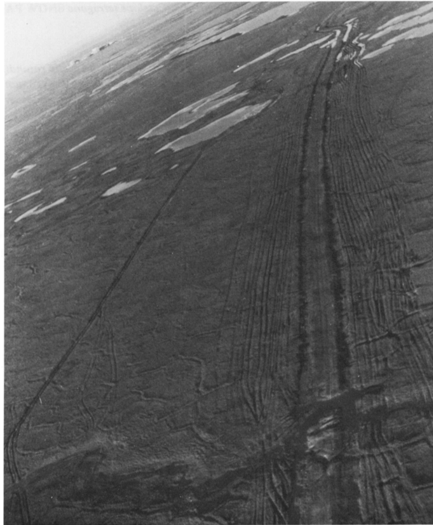
Figure 80. Deeply rutted vehicle tracks and an early attempt at road construction prior to development of the main gravel road network. Trenches on either side of the road were source of material which was bladed onto the road. Note the thermokarst across the road and in the trenches.
