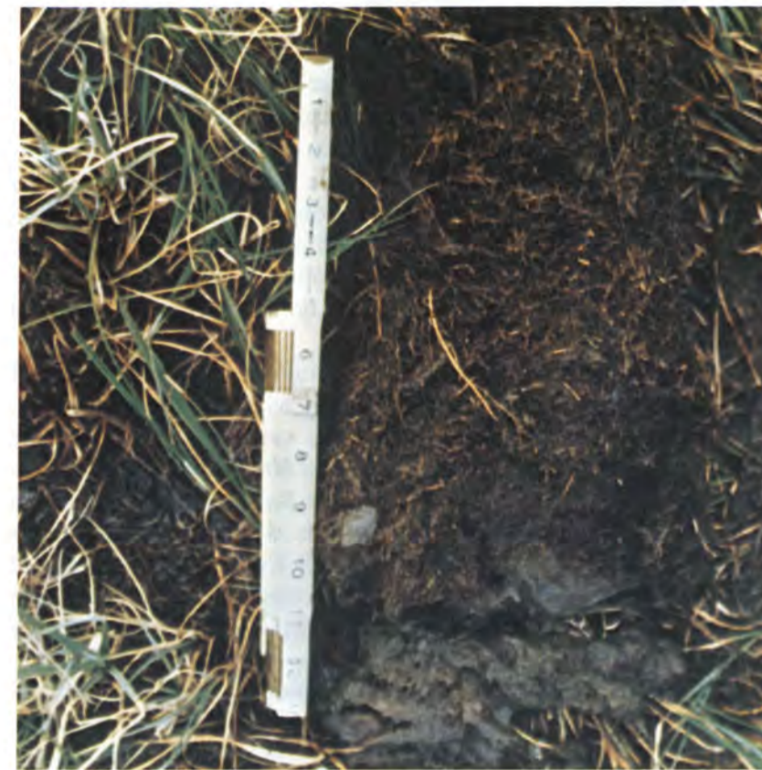
Figure 47. Units 3(1) and 4(1). These soils with thick organic surface horizons are widely distributed in the Prudhoe Bay area. They occur in the centers of low-centered polygons (Landform Units 3 and 4) and are common in Landform Units 7 and 0. Figure 43 depicts schematically the relation of this soil and that in Unit 3(2) to the Pergelic Cryosaprists (Fig. 49).
