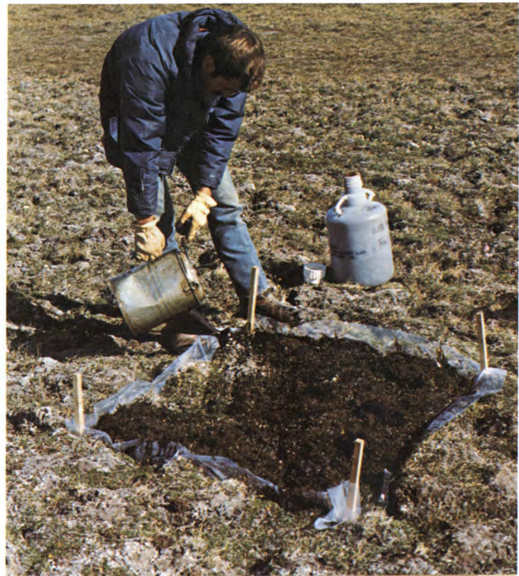
Figure 98. Experimental plot to determine terrain sensitivity to oil spills. Several similar plots were placed in the common map units.
