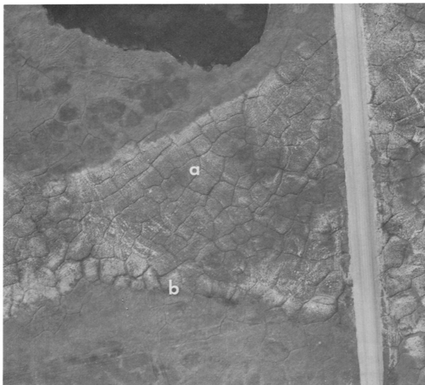
Figure 30. Unit 2. Left: High-centered polygons near the sand dunes, a) <0.5 m, b) >0.5 m. Right: High-centered polygons near the coast, with water-filled thermokarst pits in the polygon troughs.
