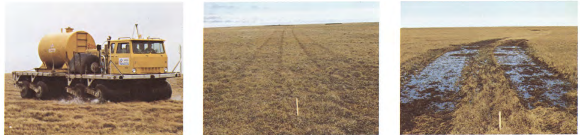
Figure 100. Off-road vehicle experiment. Left: Rolligon test vehicle weighing 11,340 kg (25,000 lb) with 0.21 to 0.35 kg/cm 2 (3 to 5 psi) ground pressure. Center: impact to an upland area, code U3/2,9. Right: impact to a lowland area, code M4,U3/4,7.
