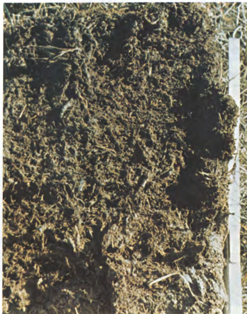
Figure 48. Unit 3(2). Such fibrous organic soils occupy very poorly drained areas or areas with shallow standing water such as the centers of low-centered polygons (Landform Unit 3). These soils occur sporadically in Landform Units 4, 7 and 0.
