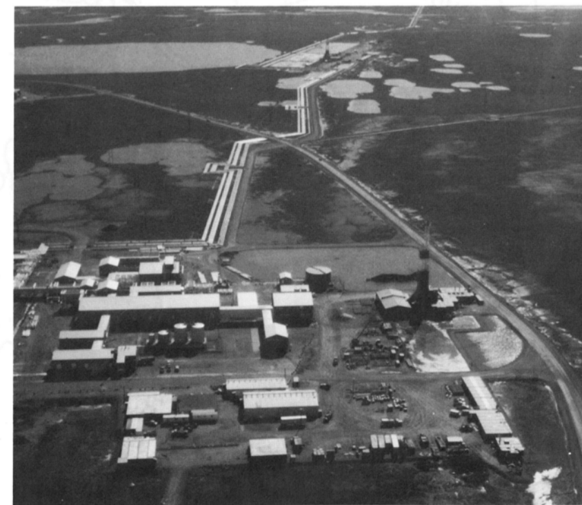
Figure 3. Oilfield facilities. Oil flows from the wellheads such as at Pad B (background) to processing sites such as G.C.3 (foreground). The spine road curves across the photograph from lower right to left. Photograph by K. Bowman.
