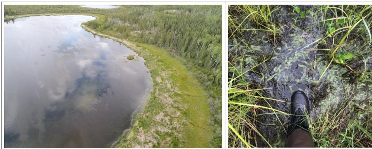
Figure 2. Left: Example UAV photo used for interpretation of inundation extent in conjunction with GPS measurements. For scale, the author is barely visible in a canoe on the right edge of the lake below the islet. Right: Field photo showing shoreline measurement method. Field teams walked along the edges of inundated areas (top majority of image) carrying handheld GPS receivers.
