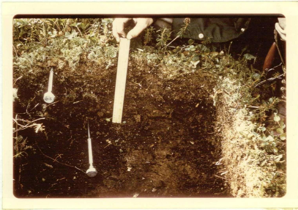
Figure 28. Tundra Moss soil (Kubiena, 1953), Meadow Tundra (Tedrow et al. 1958) associated with the Betulo - Chamaemoretum . Surface layer of living Sphagnum overlying raw humus or old Sphagnum . Depth to permafrost 27 cm. Sampled August 4/65. (Photo by Krajina)
