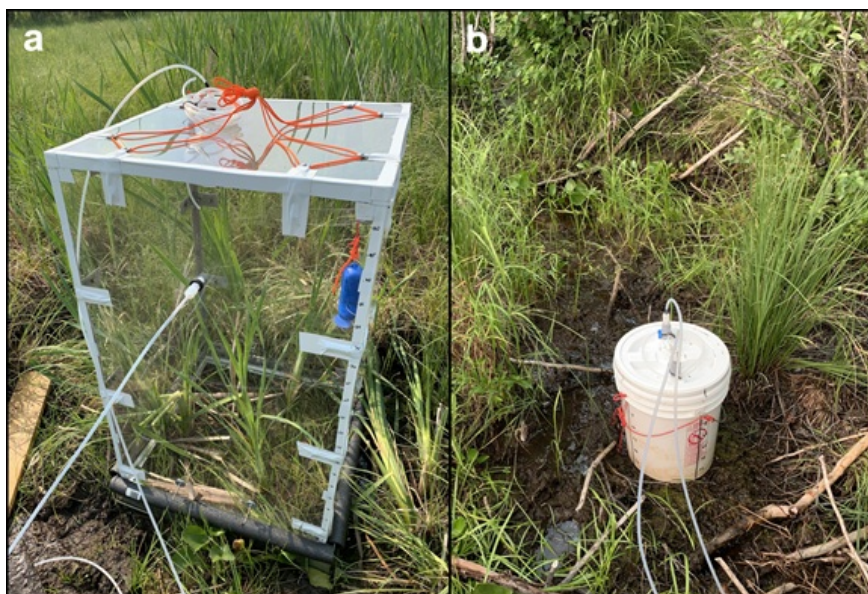
Figure 1. Chambers used to measure diffusive CH 4 fluxes. a) Large chamber resting on the pre-installed aluminum collar, sealed on edges with pipe insulation. b) Five-gallon (18.9-liter) bucket with an open bottom and air-tight screw lid to measure hotspot flux locations.
