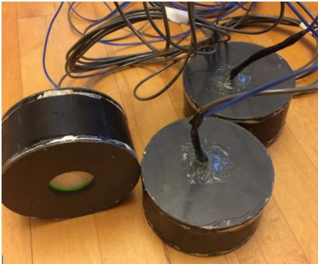
Figure 2. Soil-Depth chambers used to measure the concentration of \text{CO}_2 and temperature within the soil profile at depths of 5, 15 and 25 cm.
